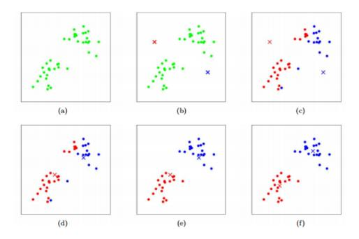
Figure 2.11: Convergence process of a k-means algorithm with k=2
