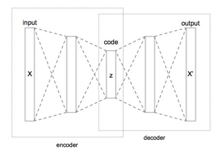
Figure 2.8: Abstract layers of an Autoencoder model where the model tries to reproduce the input through an intermediate dense representation.
