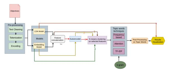
Figure 5.1: A Block diagram of the methodology used in this study. An objective document is passed through a Pre-processing step first, then one of five type of feature spaces is selected which is used of clustering. Next, one of the three topic word retrieval technique is selected to get the top topic words. Last step is post processing to remove redundant topics from clusters.
