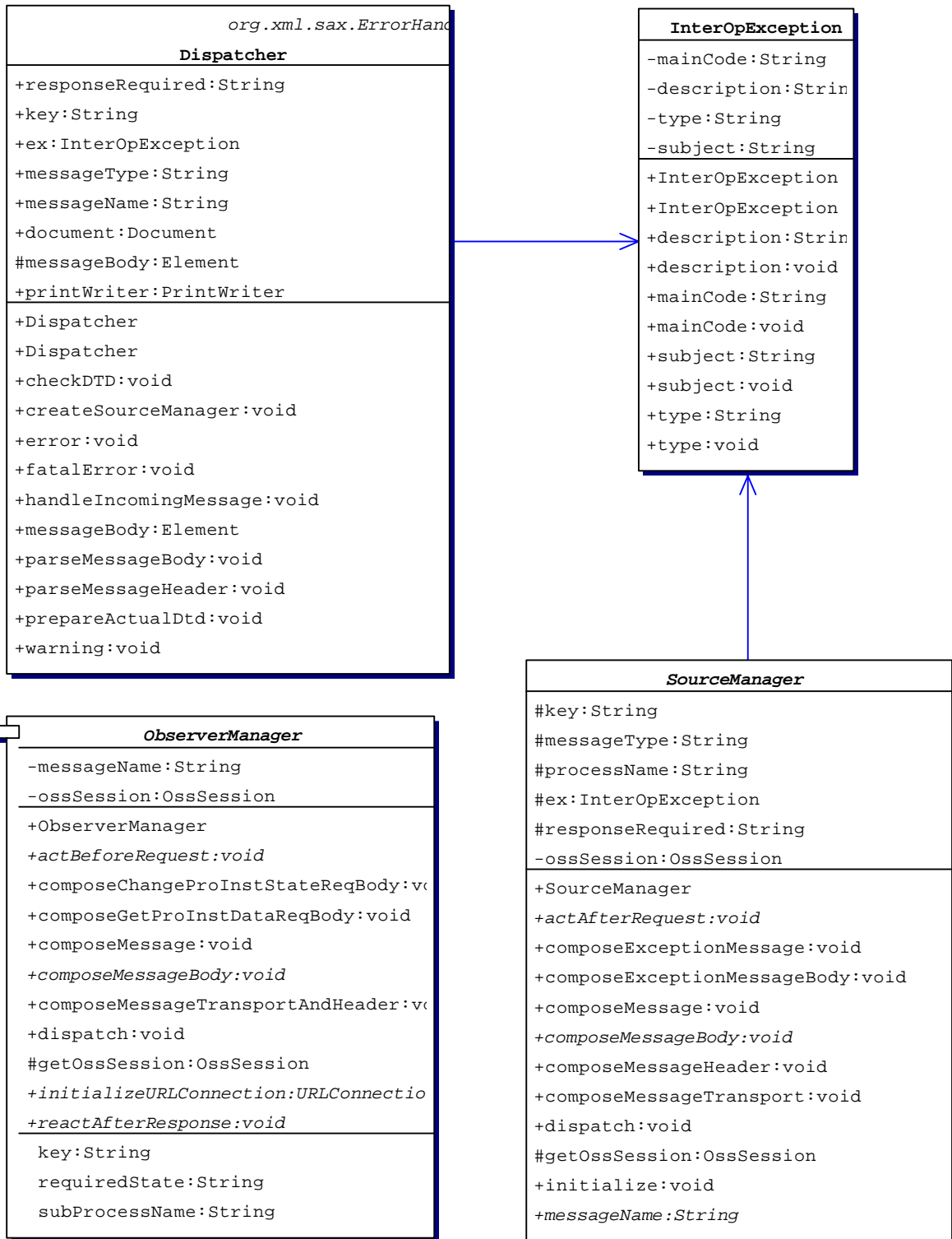
Figure 5.3: Interoperability Classes (package: de.nova.ezn.wapi.interoperability )
