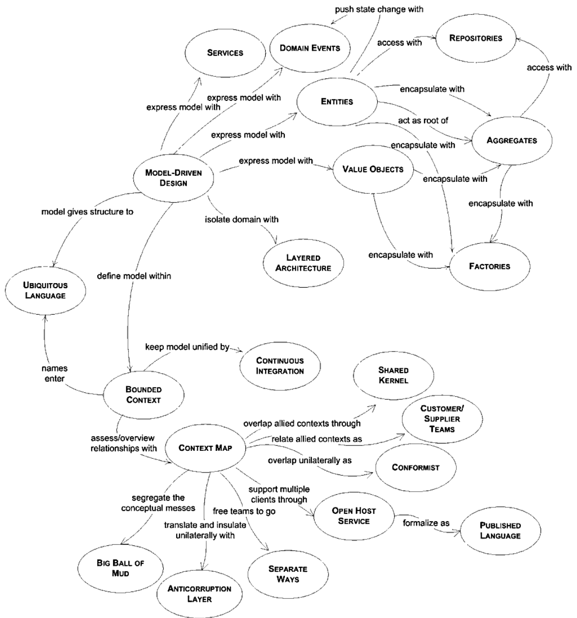
Figure 2.6: DDD Building Blocks and Context Mapping [31]
